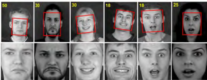
Fig 7. Results obtained by the proposed tracker on key frames taken from sample videos of MMI and MUG facial expression database under head rotations and varying expressions (upper row). Images on the lower row show cropped faces with rotation corrected face geometry.
